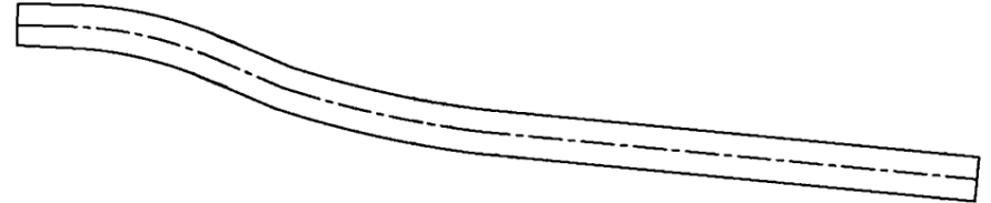
27x17 oval tapered to 16mm round single bend
