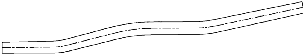
19mm round tapered to 16, both ends
